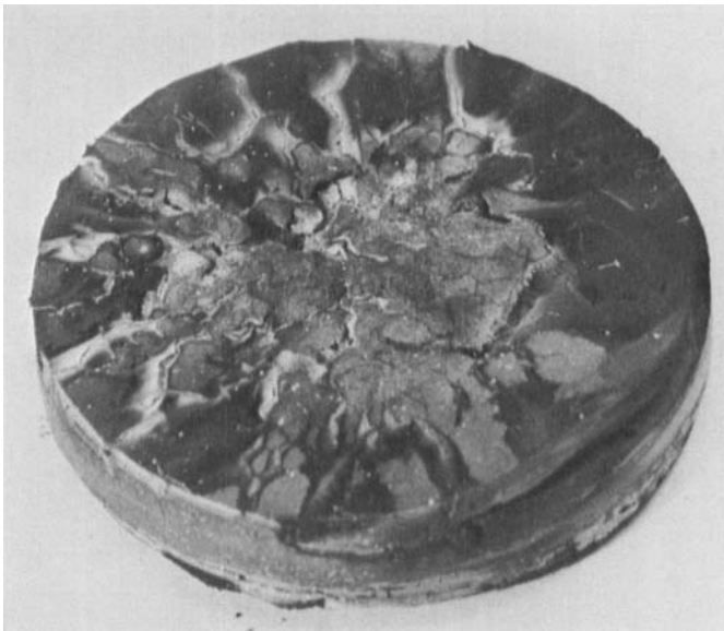
Fig. 12. Oxyacetylene torch test, sample N-34 (4.2% Cl, 1.83 C/H + Cl) + 4 pph chopped quartz fiber, uncured.
