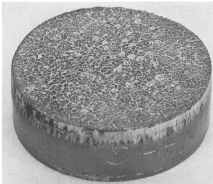
Fig. 13. Oxyacetylene torch test, sample N-44 (4.6% Cl, 187 C/H + Cl) + 4 pph chopped quartz fiber, cured.
