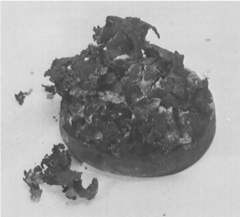
Fig. 11. Oxyacetylene torch test, sample N-1 (0.8% Cl, 1.50 C/H + Cl) unfilled, uncured.
